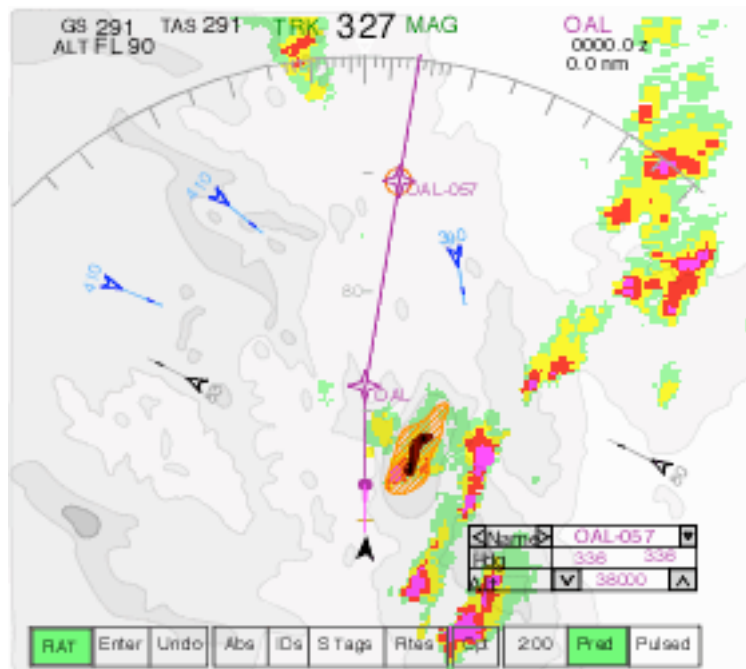
Fig. 5. Integrated cockpit display of navigation information and traffic, weather, and terrain hazards. Nonhazardous terrain and weather have low luminance-contrast to prevent distraction from critical information. Terrain hazard is distinguished from weather hazard by texture.
